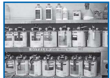
Storing/keeping all solvent containing materials in closed containers
